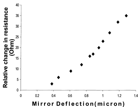
Fig. 10. Mirror deflection vs. relative change in resistance of a single piezoresistor.
